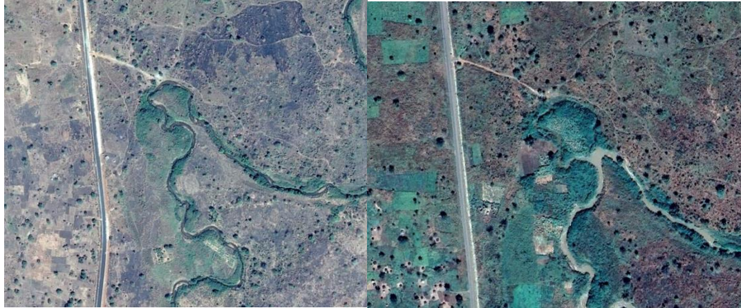
Figure 2.18: Left: February 2016 where The outer bend of this river experiences soil erosion as a result of the high flow velocities in the river. Right: October 2018 where the bend becomes isolated from the river resulting in a horseshoe lake
